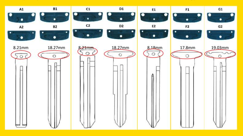
Directions: To determine which adaptor to use. Remove and measure the key head width (circled) and match your key to picture. Fit corresponding adaptor. Change over electronics from broken shell into new shell. Assemble and screw together.
